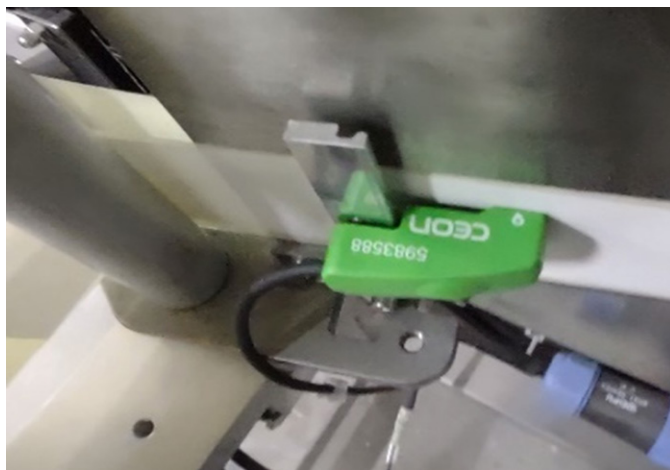
Fot. 1. Label sensor mounted on the measuring station
