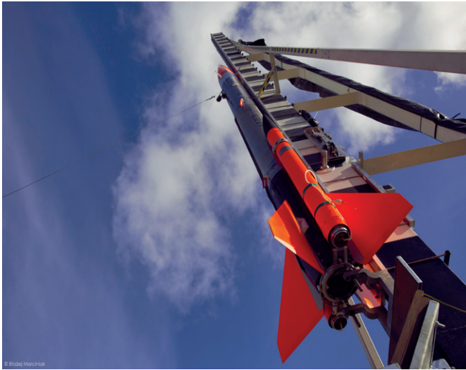
Fot. 5. Rocket ILR-33 BURSZTYN ("AMBER") – the first rocket in the world, employing hydrogen peroxide above 98% as antioxidant. The project was initiated by Prof. Piotr Wolański. Photo. Błażej Marciniak. Source: Łukasiewicz – Aviation Institute
