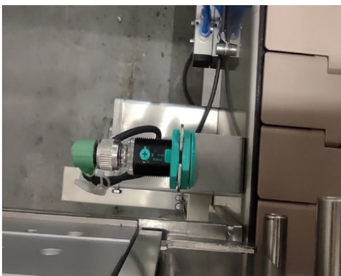
Fot. 3. Product sensor mounted on the measuring station
