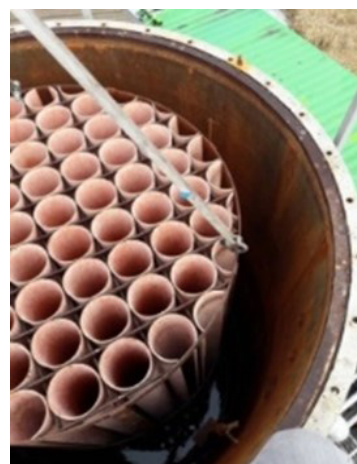
Fot. 1. Pilot biogas plant: a) site of biogas plant (a view [Photo by G. Wałowski] – from right: fragment of pig house, mono substrate flow reactor for methane fermentation of pig slurry together with the installation for production of agricultural biogas, lagoon for post-fermentation product; b) adhesion bed, made from vertical pipes with coarseness of 80 μm, transported to the inside of fermentor – a view [Photo by G. Wałowski].
