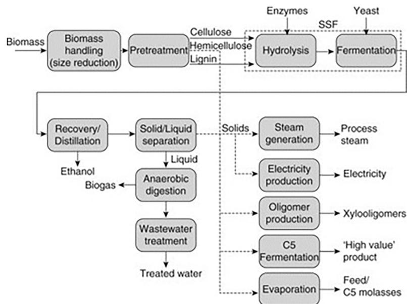
Fig. 6. Conception of "energy-driven" bioethanol-based biorefinery [33]
