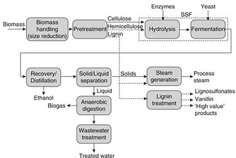
Fig. 5. Conception of "C5-driven" bioethanol-based biorefinery [33]
