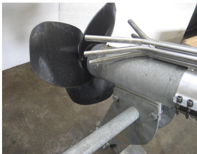
Fig.4 Detailed view of acid discharge system of ORUM Co. – construction of "in storage" unit
