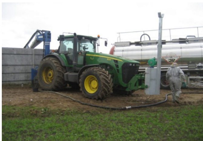
Fig. 3. Orum Smeden's "in storage" acidification system at work Source: Orum Semden's marketing material
