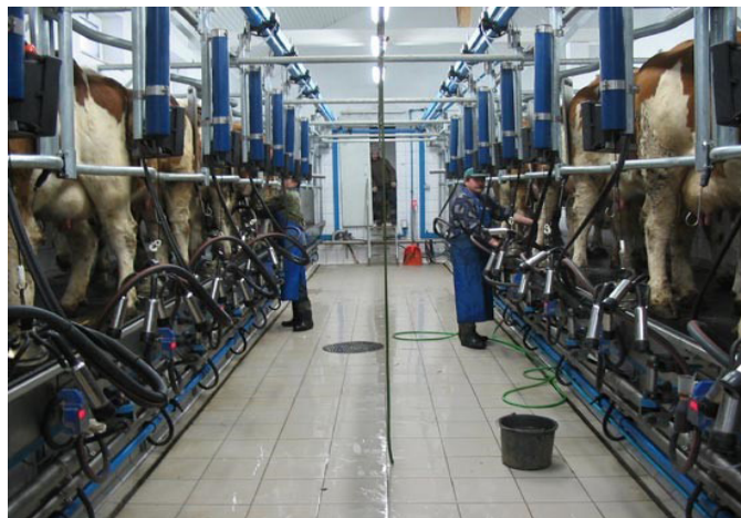
Fig. 2. Milking parlour of „herringbone“ type [24]
