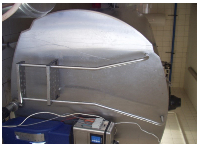
Fig. 4. Cooling tank for milk [photo made by the employees of the Institute]
