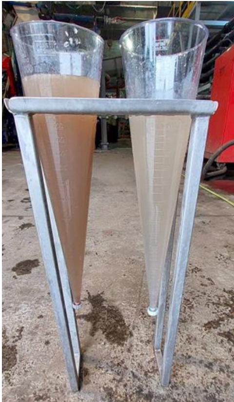
Photo 1. Comparison of effluent samples – raw effluent (left) and effluent after phase separator (right)
