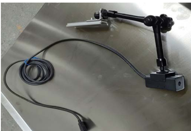
Photo 2. Camera mounted on the articulated arm
