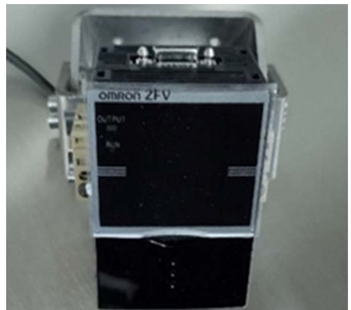
Photo 3. Camera setting panel assembled with adjustable mount
