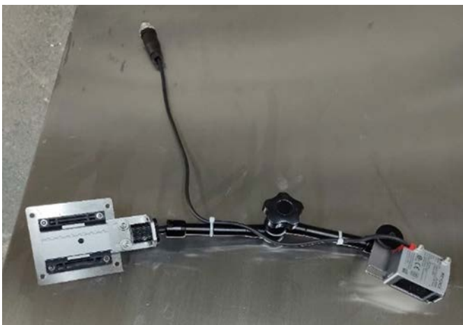
Photo 1. Sensor mounted on the articulated arm
