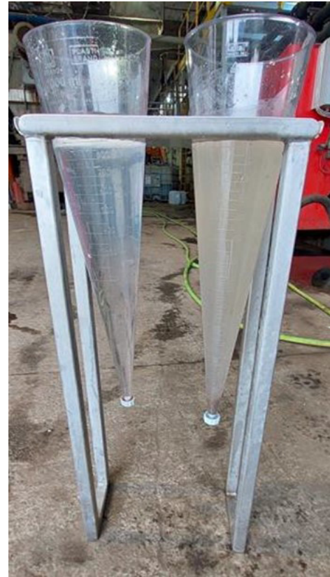
Photo 2. Comparison of effluent samples – effluent after membrane filtration (left) and effluent after phase separator (right)
